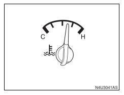
Your vehicle is equipped with an engine coolant temperature gauge. With the igni-
